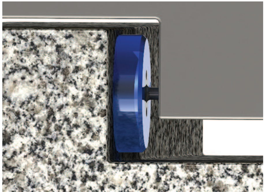
90mm vacuum Preloaded Air Bearing Application 3-D Model
