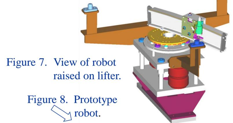
Figure 7. View of robot raised on lifter.
