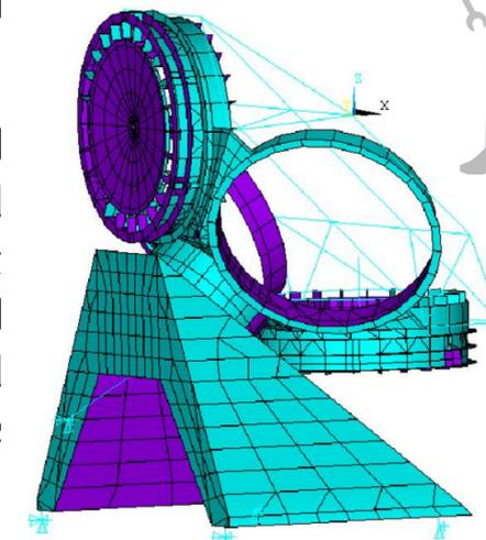
Figure 3. FEA model of exchanger created to check dynamic performance and stresses under earthquake loading.
