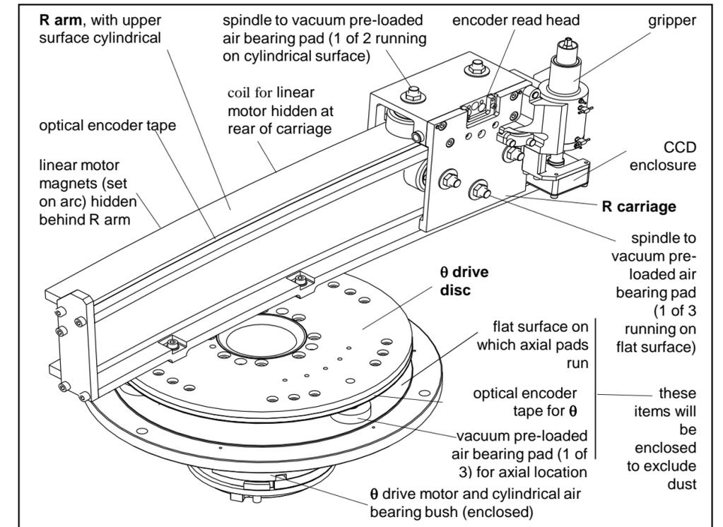
Figure 6. Details of R-θ robot.
