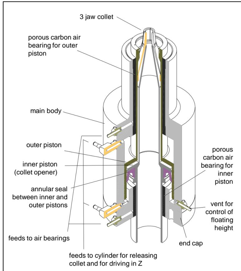
Figure 4. Section through gripper assembly with main components identified.
