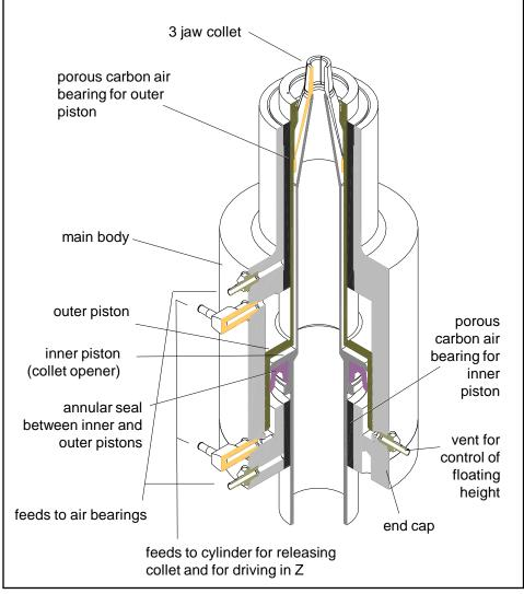
Figure 4. Section through gripper assembly with main components identified.
