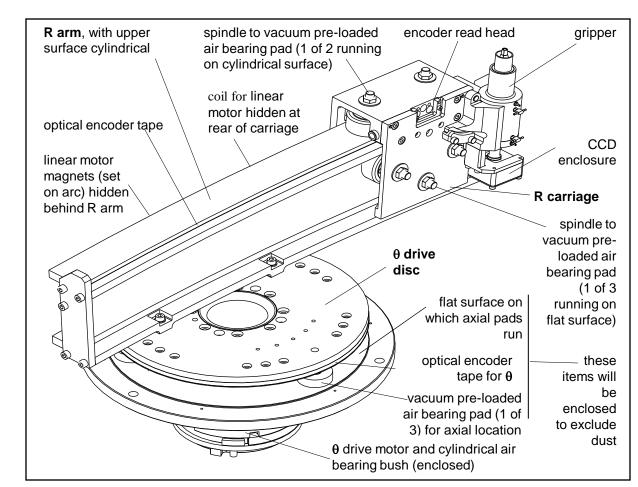
Figure 6. Details of  $R-\theta$  robot.
